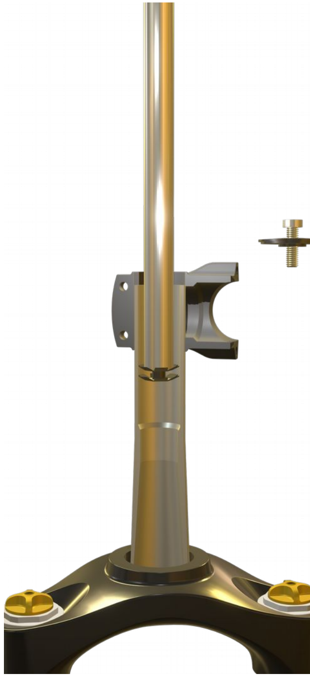
Figure. 2: Removing the star nut
