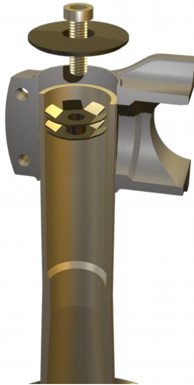
Figure. 1: Unscrew star nut from the top of steerer tube
