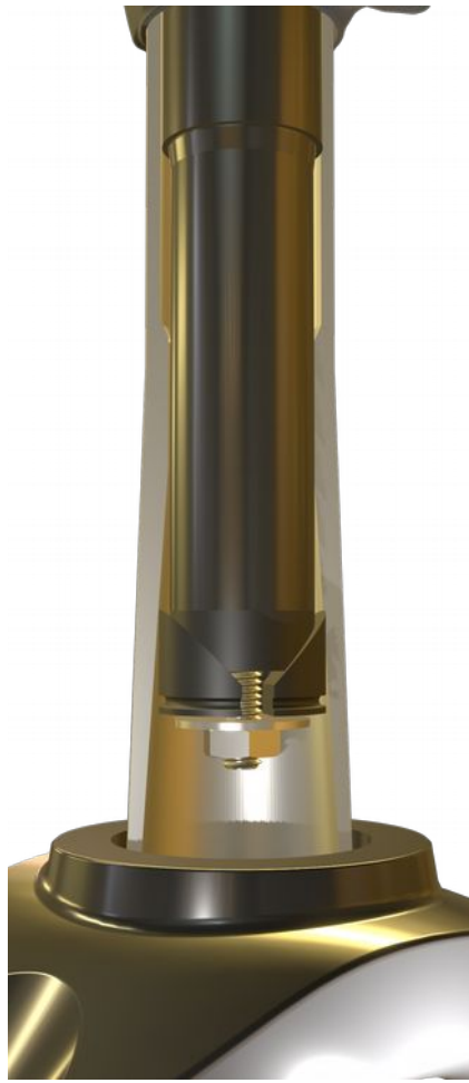
Figure 5: Tightening the screw from the bottom
